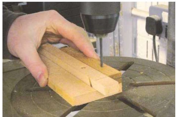
▲ Pic.4 With the metal and wood piece held together, he drilled holes for the brass rods
